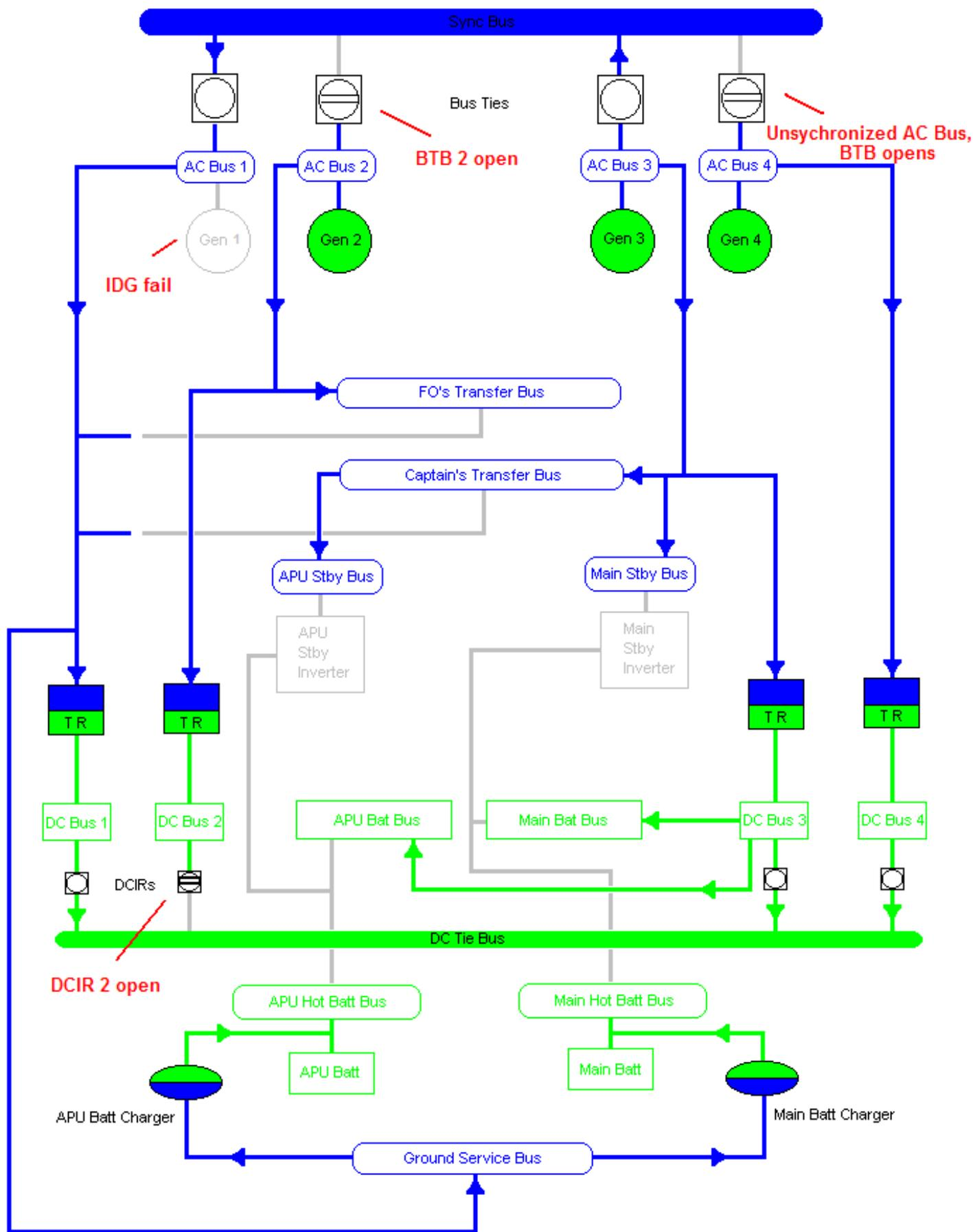
**Electrical faults: IDG Fail, BTB open, DCIR open, and Unsynchronized AC Bus**
