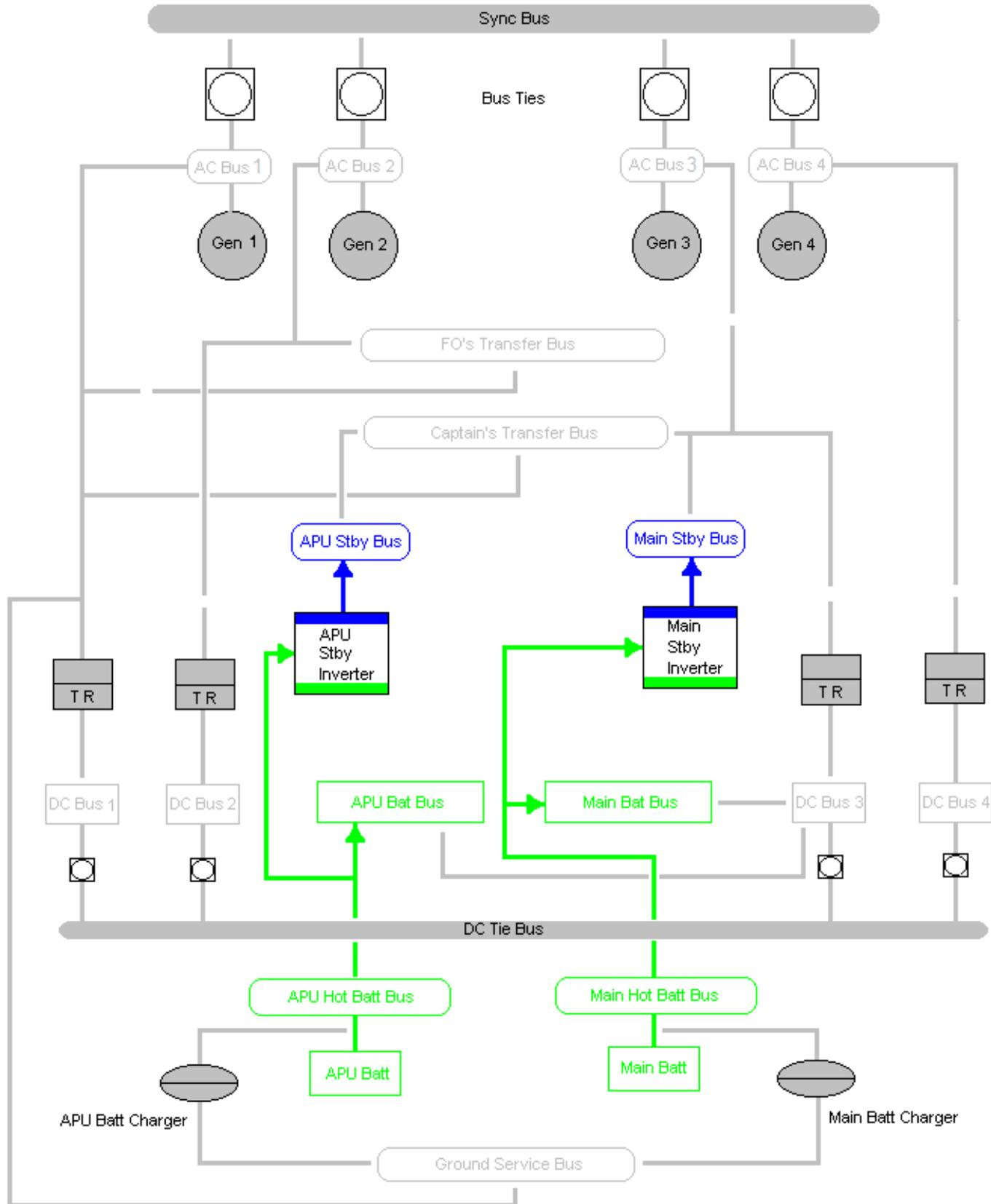
**Electrical faults: All generators failed**
