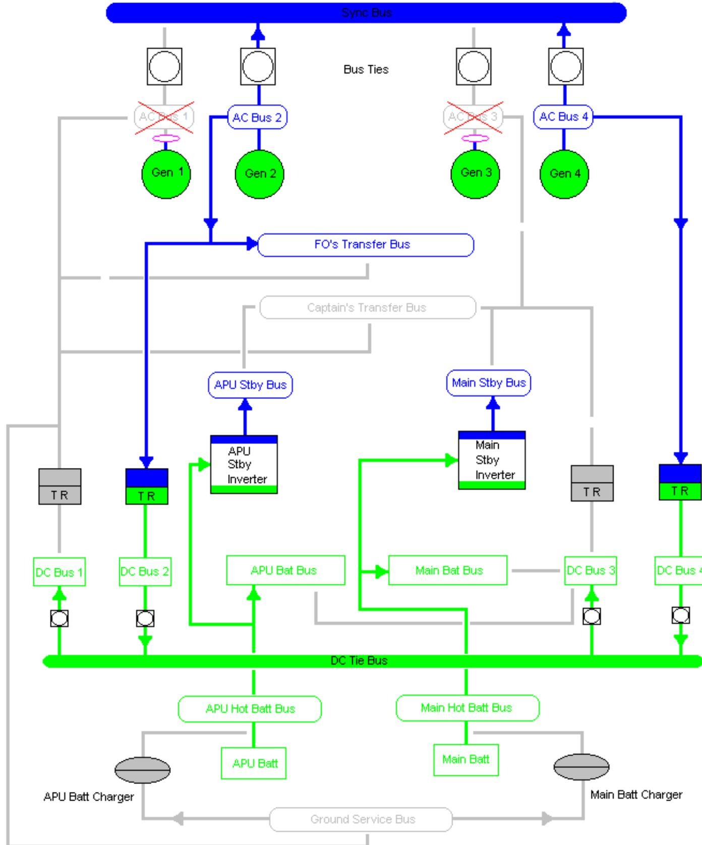
**Electrical faults: AC Bus 1 and AC Bus 3 failed**
